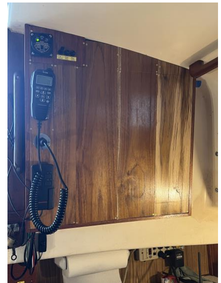
Figure 14: Interior cabinet covering the back of the new instruments and wiring.
